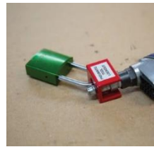
Fig. Error! No text of specified style in document..4 Pneumatical Lock-out system
