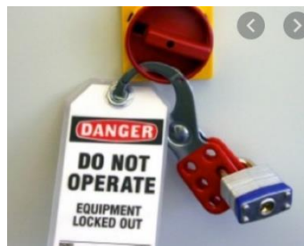
Fig.4. Electrical Lock-out system
