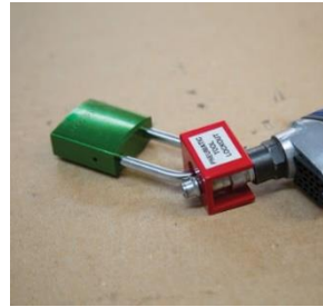
Fig.5. Pneumatic Lock-out system
