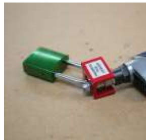
Fig.5. Pneumatic Lock-out system
