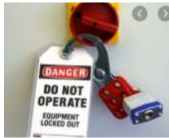
Fig.4. Electrical Lock-out system
