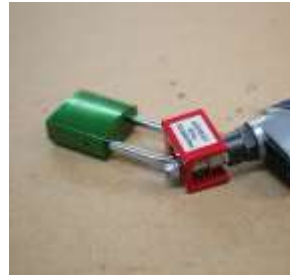
Fig.5. Pneumatic Lock-out system
